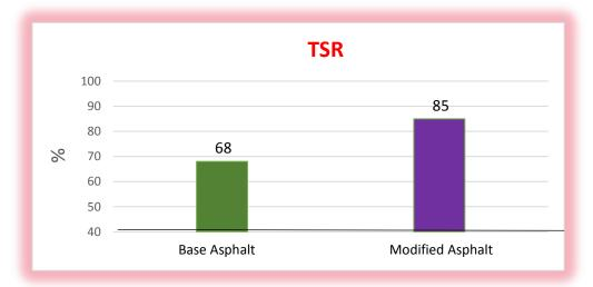
Tensile Strength Ratio (TSR) Must be more than 75%
